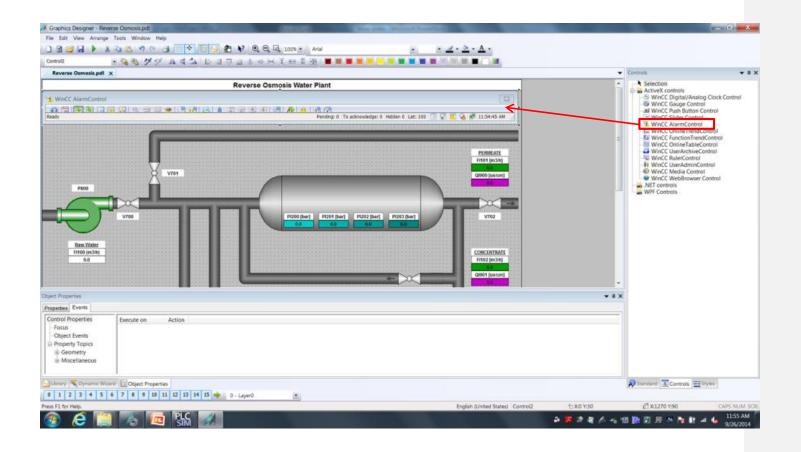
10. We're going to clean up our Alarm Control a little. In the "WinCC AlarmControl" view of the object configuration dialog window, make the settings below:
