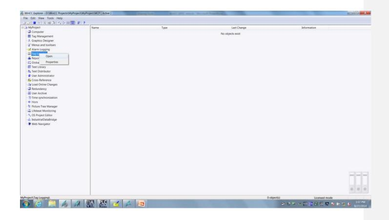
2. In the WinCC Configuration Studio Tag Logging, click on the **process value archiving** and create a new archive by typing the name in the column.
